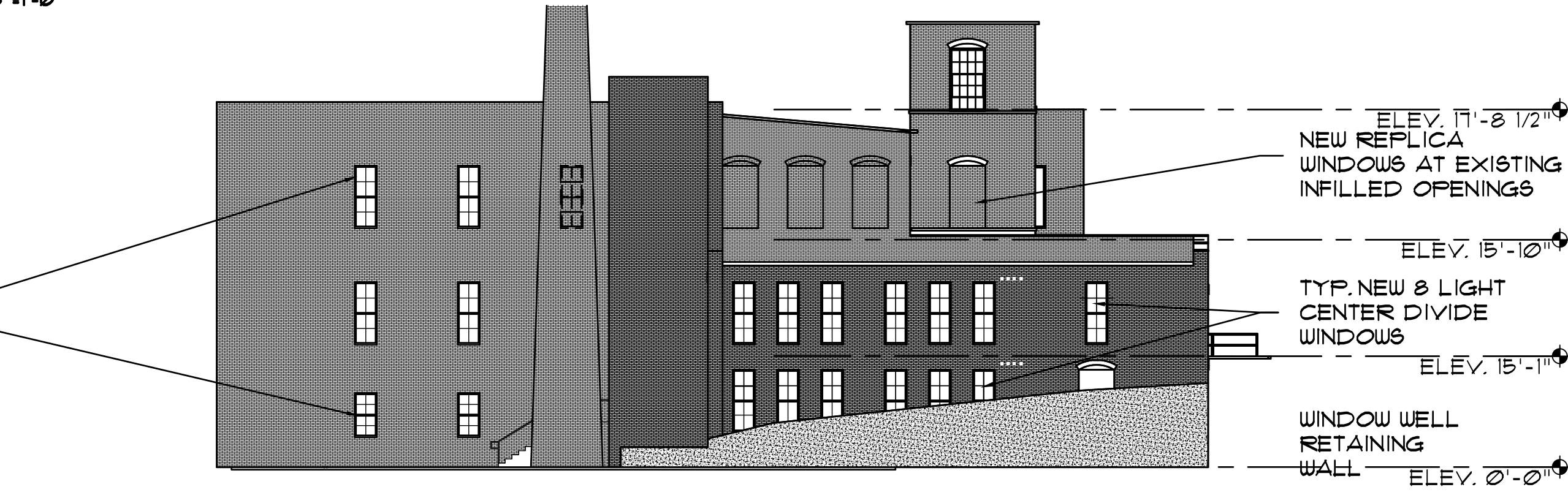
2 MAIN MILL NEW SOUTH ELEVATION 1/16"=1'-0" East Elevation
